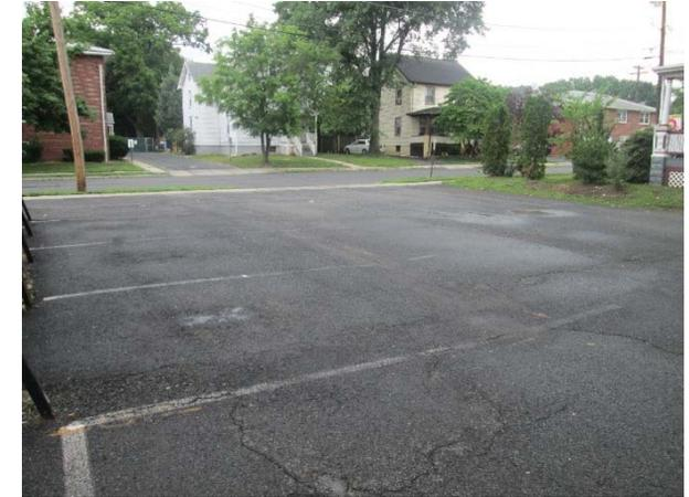
Parking lot runoff currently flows toward the street. The parking lot can be partially redone with pervious pavement to capture this runoff as well as some of the roof runoff. The building has disconnected downspouts, which can also be directed into two bioretention systems in order to capture, treat and infiltrate runoff. A preliminary soil assessment for this site suggests that soils have suitable drainage characteristics for green infrastructure.
