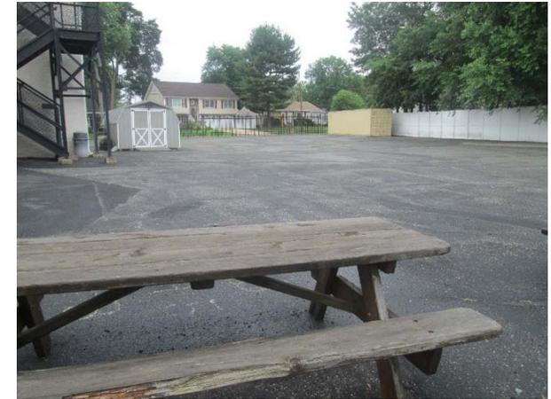
Community Bible Church has a roof with disconnected downspouts and a large paved area. A bioretention system can be built at the front of the building to capture, treat and infiltrate runoff. The large paved area and some roof runoff can also be treated with pervious pavement. A preliminary soil assessment for this site suggests that soils have suitable drainage characteristics for green infrastructure.
